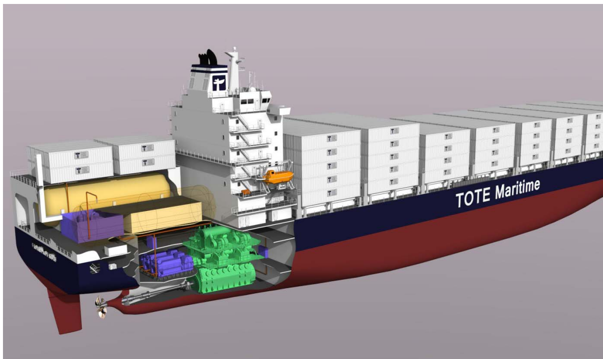
Container Ship powered by MAN 2-stroke Dual Fuel engine ME-GI
